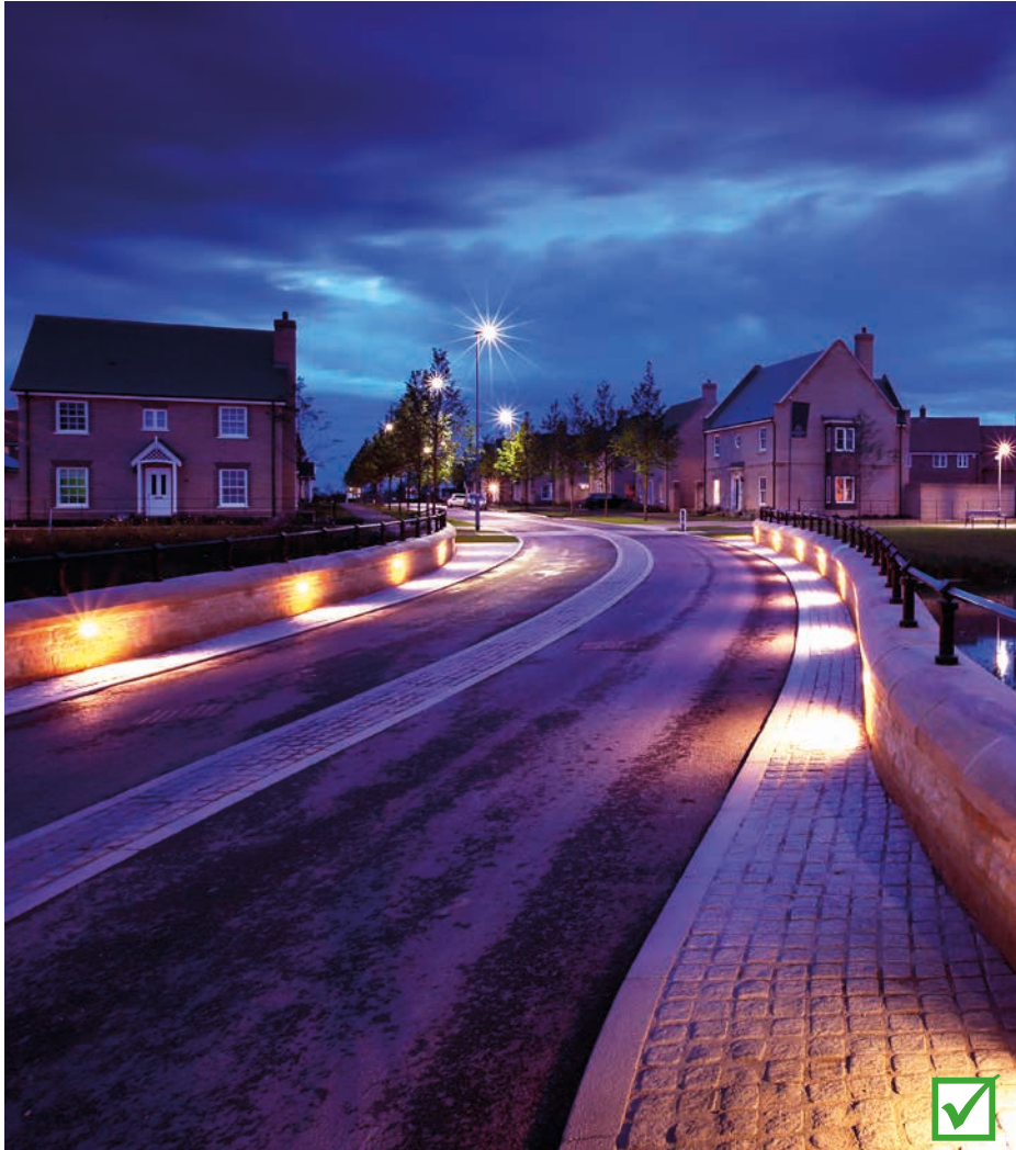
Integrated downlights are used to avoid clutter on the street
